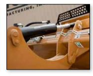
Anti-Rotational Pins & Cross Tube Cylinders
