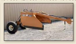
**Side Supports:** Tapered and beveled for extra strength and durability
